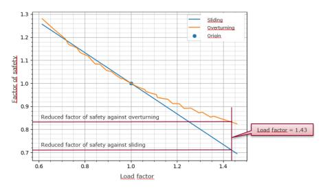
Figure 9. Computed correlation between load factor and factor of safety with changing pore pressure. Origin represent å linear pore pressure from upstream to downstream side.
