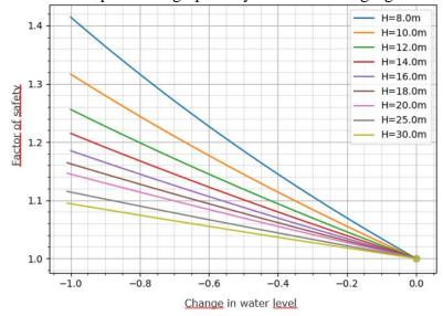
Figure 4. Sliding: Reduced water level vs. factor of safety for different dam heights.
