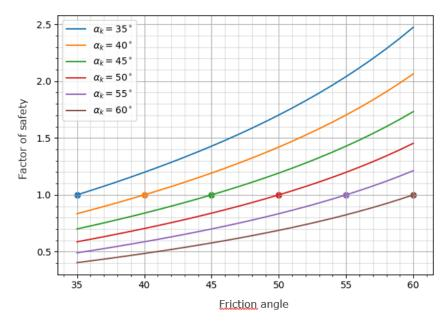
Figure 3. Correlation between factor of safety and friction angle.  $\alpha_k$  is the initial friction angle where the dam cross-section have factor of safety = 1.0.
