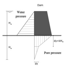
Figure 1. Illustration of assumptions to generate pore pressure.
