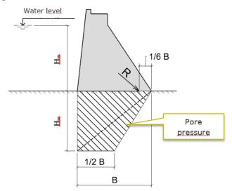
Figure 8. Maximum allowable pore pressure assumed for accident loads. Pore pressure distribution for normal design loads is shown as a dotted line.
