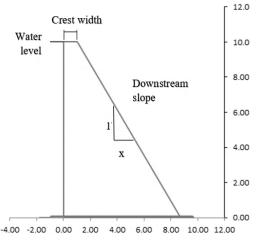
Figure 2. Dam section is selected by varying crest width and downstream slope.
