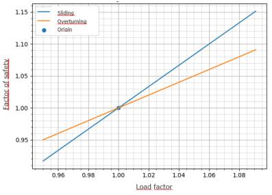
Figure 7. Load factor vs. factor of safety (Friction angle =  $40^{\circ}$ )
